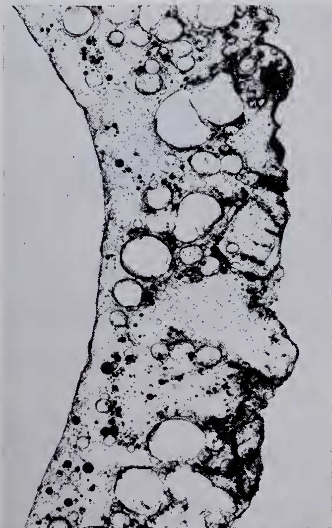
Figure 3.—Photomicrograph of thin section of fulgurite from Willetton. The smooth inner surface is on the left, and contrasts with the rough outer surface on the right. Large vesicles tend to be elongated normal to the lumen, and small bubbles show up as almost solid black circles. Length shown = 2 mm.
